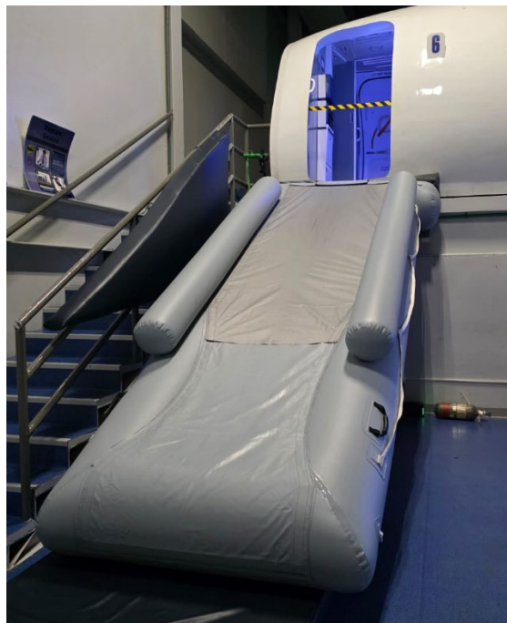
Figure 1: Installed Single Lane Evacuation Training Descent Slide
