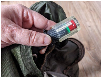
Figure 28 - Manual mode conversion - Steps to change the inflator cap
