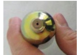
Figure 22 - Pierced / Used cylinder
