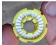
Figure 26 - (Image 1) - Opening for the bobbin on the inflator / (Image 2) Salt Tab Bobbin / (Image 3) Armed inflator in automatic mode
