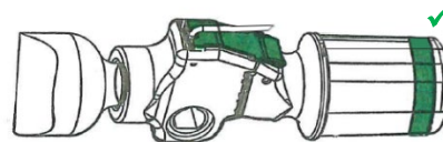
Figure 26 - (Image 1) - Opening for the bobbin on the inflator / (Image 2) Salt Tab Bobbin / (Image 3) Armed inflator in automatic mode
