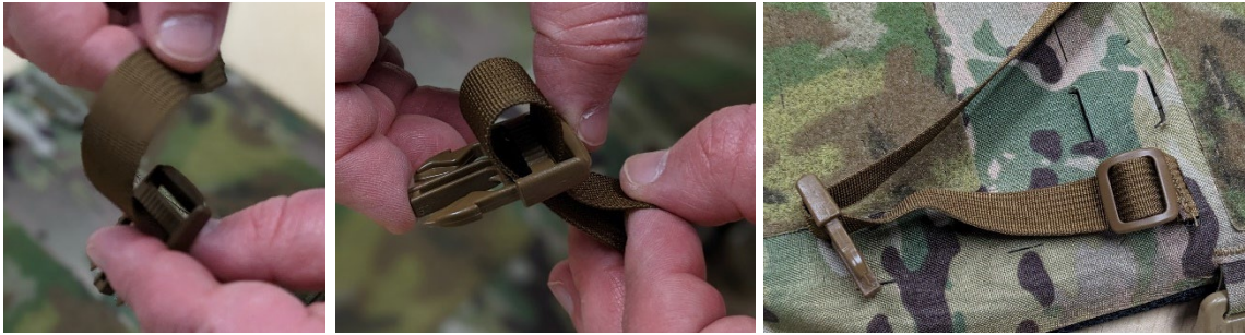
Figure 13 - Steps to weave the male buckle back on the strap
