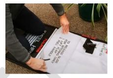
To reset the inflate simulation side, hold the plate assembly base firmly, and place the flat end of the magnet back on the open circle, until the magnet clicks back in place. Place the red pull handle back on the Velcro area.
