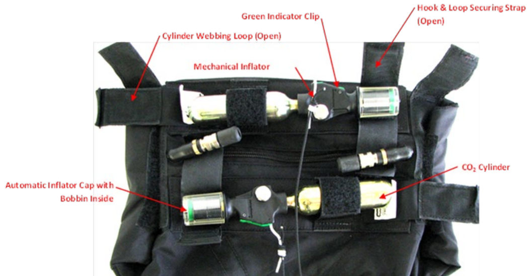
Fig 2.5: Mechanical Inflation System
