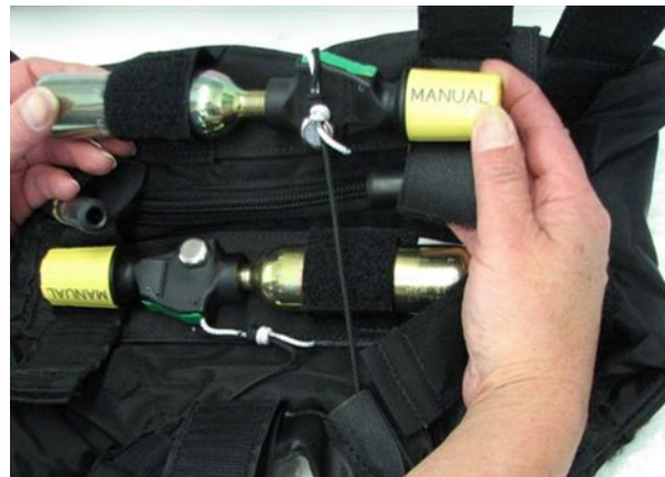
Figure 3.15: Installation of Manual Mode Cap
