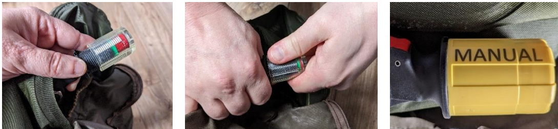
Figure 28 - Manual mode conversion - Steps to change the inflator cap
