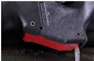
Figure 23 - Closed red inflator lever
