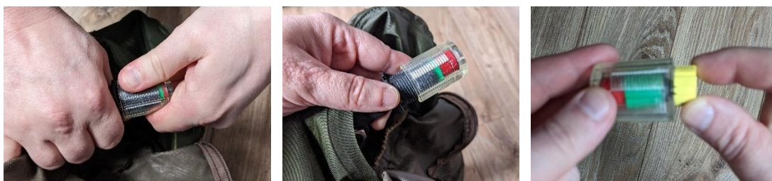
Figure 25 - (Top) Bobbin expiry date / (Bottom) Steps to remove the bobbin
