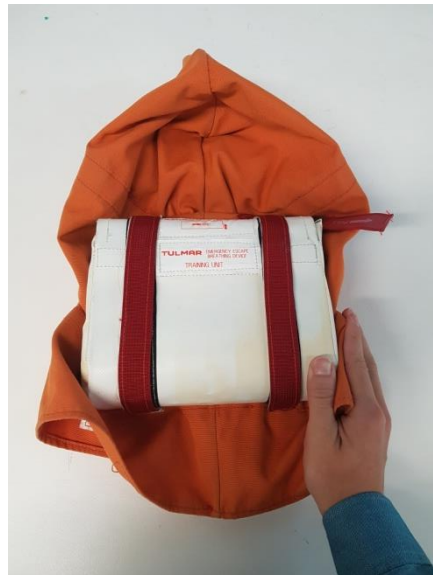
Figure 6: Folding sides of PBE inwards
