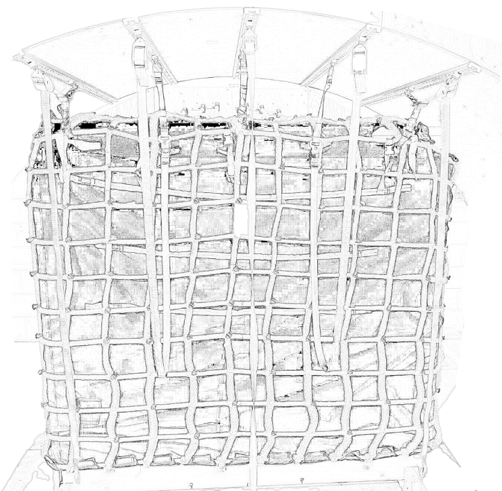
FIGURE 12 Fully Installed and Deployed Cargo Net
