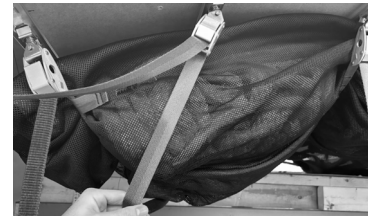
17.6 Position straps 89102-003 (these are between the corner straps and central strap) out around the baggiest parts of the package, then tighten as much as possible.
