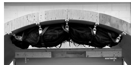
17.9 Tighten between straps 89102-003 as much as possible. Tuck loose straps and loose mesh away as needed.
