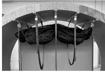
17.2 Tighten corner straps 89102-002 to match center strap 89102-004.
