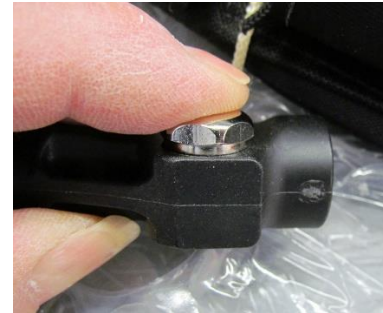
Figure 5, Seating the O-ring
