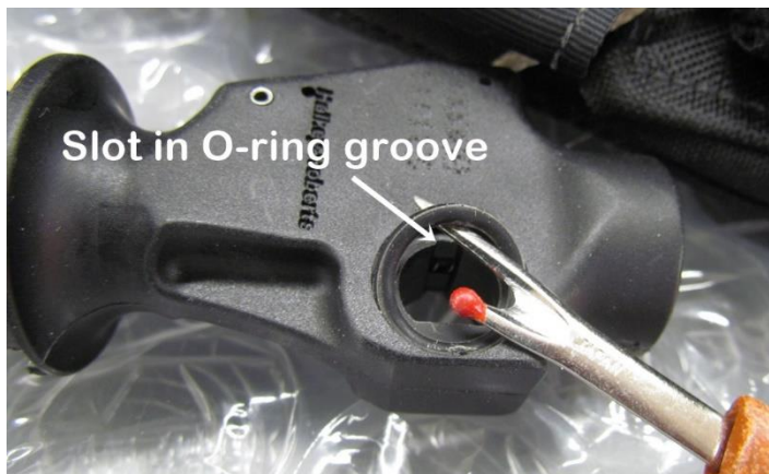
Figure 2, Removal of the O-ring
