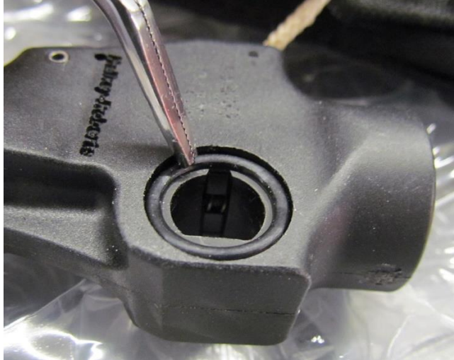
Figure 4, Inserting a new O-ring
